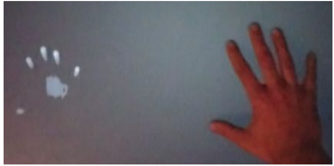
Figure 2: The user shadow (left) is a contact image captured by our surface that we display at an offset from the user’s hands
